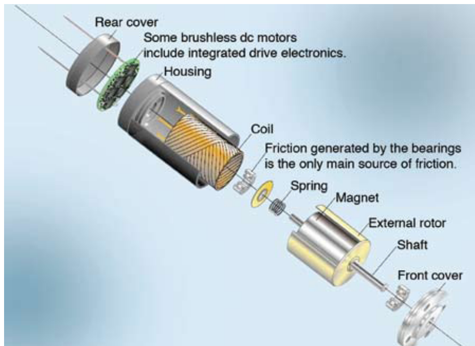
Figure 2.1: A BLDC schema [1]
