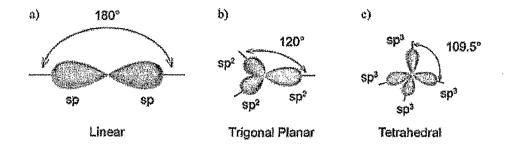
Figure 1.1: The different hybridisations of carbon a)  $sp^1$ , b)  $sp^2$ , c)  $sp^3$
