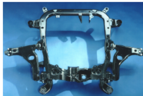
Engine frame with mounted parts
