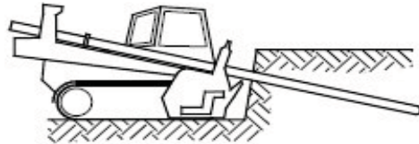
STEP 2. DRILL NAIL HOLE
