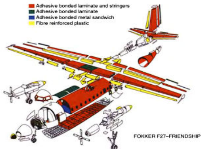
Plate 1: Many aircraft parts are bonded with high performance adhesives, on this FOKKER F27 as well as on the Airbus A380.
