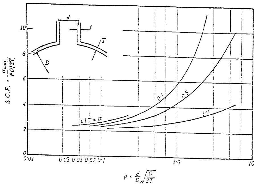
Approximate stress concentration factors in flush nozzle reinforced openings in cylindrical shells.
